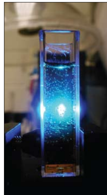
The lab of Craig Hill, above, led the project. At right, bubbles of oxygen form from water oxidation, catalyzed by the new tetra-cobalt WOC.
