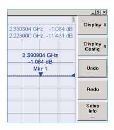
Context-sensitive help including detailed description of the active function and display of the associated remote-control commands supports also untrained users and simplifies programming
