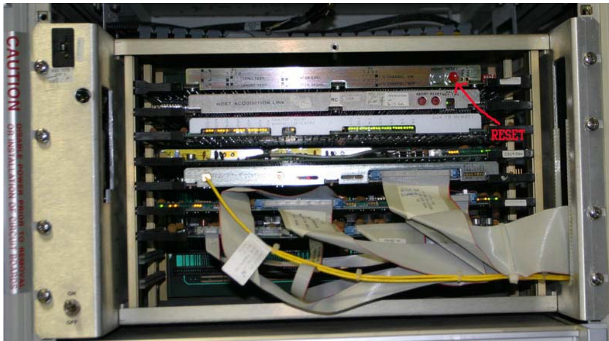
UNITY600 Plus Console RESET button position.
